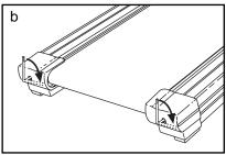
mill for a few minutes. Repeat until the walking belt is properly tightened.
